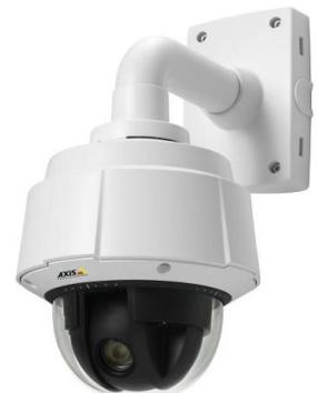
Arctic Temperature Control allows the camera to not only function at -40°C (-40°F) but also power up at that temperature following a power failure. AXIS Q6032-E can operate in temperatures from -40°C to 50°C (-40°F to 122°F). It has an IP66-rated protection against dust and water.
